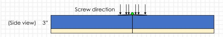
IMPORTANT: Make sure the hinge is centered over the line between the sections and the hinge flaps are parallel along the top of the wall board.
