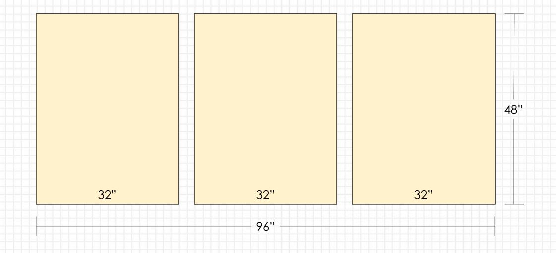
Have the sheet of plywood cut into three (3) equally-sized sections: 32" x 48"
