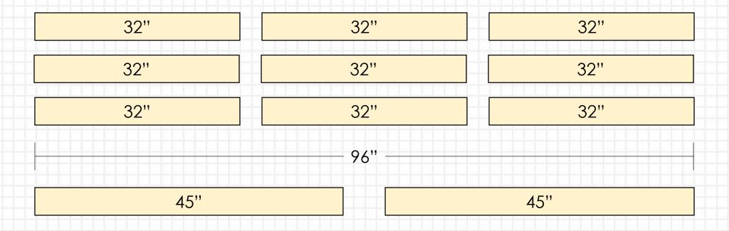
Have the four (4) 2"x 3"x 8" boards cut into lengths as shown.
