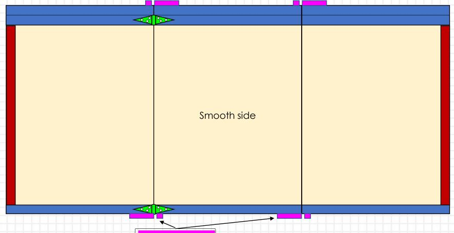
Attach four (4) slide bolts across seams between sections using the screws provided.
