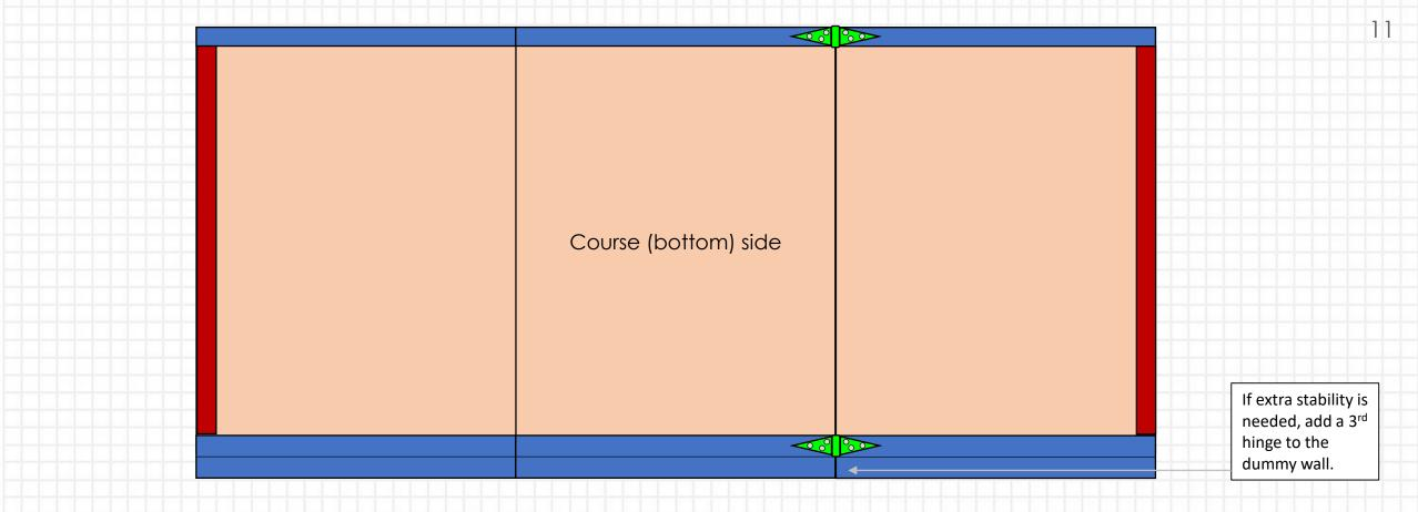
Flip over the table, push the remaining sections together so they are flush. Attach strap hinges on bottom of the walls using six (6) 1" wood screws per hinge.
